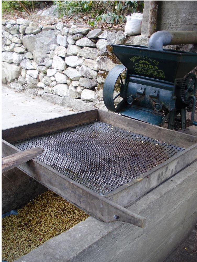
Manual coffee berry pulping machine from Peru. The beans in the basket have been depulped already. (credit: C Schwab)
