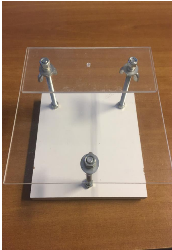
Figure 11: The home-made microscope is ready
