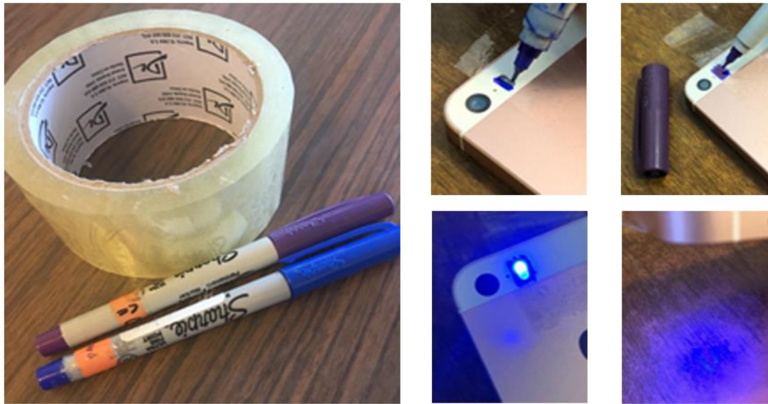
Figure 15: Materials and step by step of making a UV filter.
