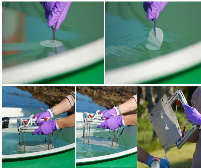
Membrane (top images) and mesh screen (bottom images) sea surface microlayer samplers.
