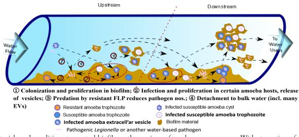
Materials and conditions to control biofilm-pathogen issues from human exposures. With stagnation of water flow, disinfectant concentrations fall, water temperatures may rise and biofilms grow along with free-living protozoa (FLP, particularly amoebal hosts to various saprozoic pathogens such as *Legionella* spp.). Subsequent water flow and aerosolization near humans may then provide an infectious dose. Adapted from Shaheen *et al.* (2019) *Int J Hyg Environ Health* 222: 678-86.
