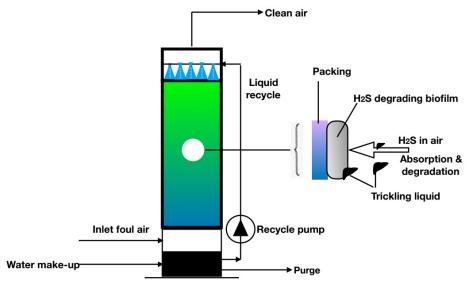
Fig 1: Summary scheme of a bio-filter in which micro-organisms grow on a carrier and convert the gaseous compound,  $H_2S$ , to sulfur powder.
